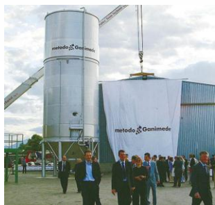
The largest Ganimede® fermenter worldwide: 15 metres high, 5 metres wide, with a capacity of over 2,000 hectolitres
